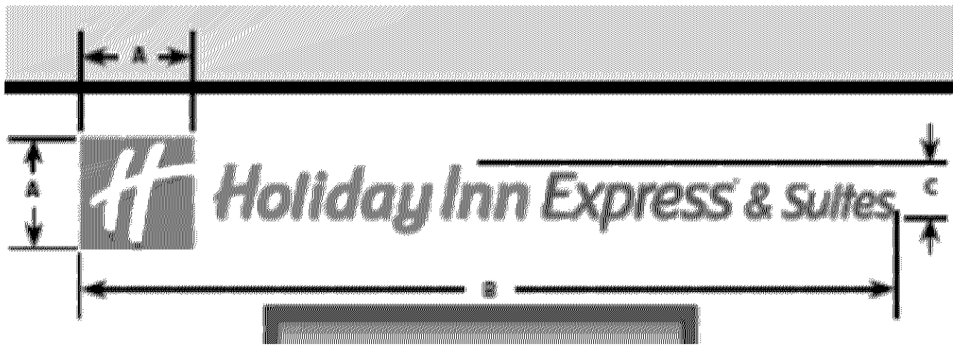
LARGE STRAIGHT WALL SIGN (DLS-LM-6) SIGN AREA = 126 SF (ALLOWED 250 SF MAX) HEIGHT TO TOP OF SIGN = 12'-0" SIGN DIMENSIONS: A = 12'-0" B = 12'-0" C = 12'-0"
