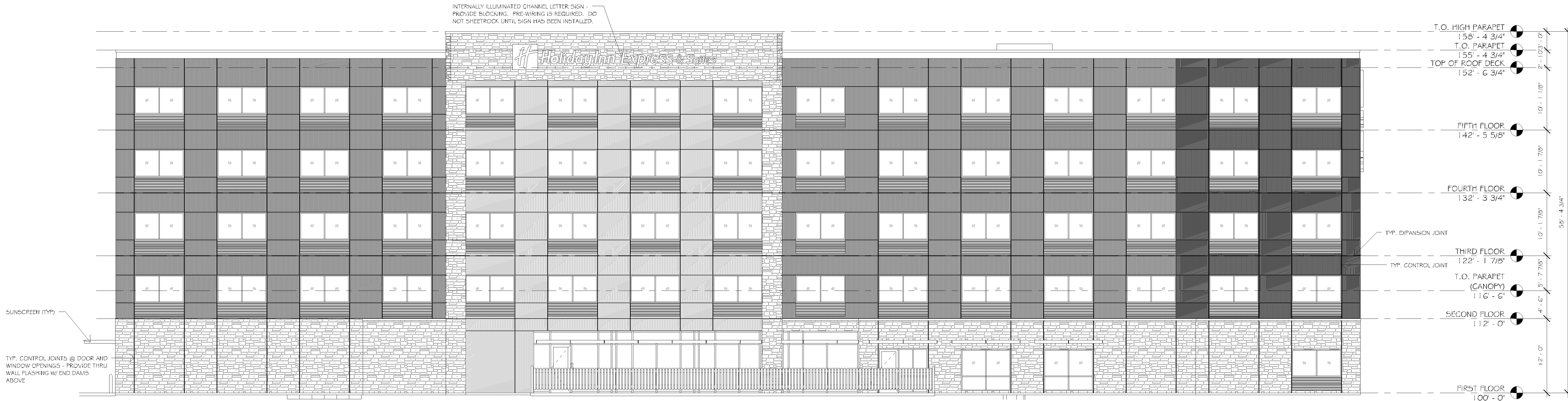
1 NORTH EXTERIOR ELEVATION SCALE: 1/8" = 1'-0"
