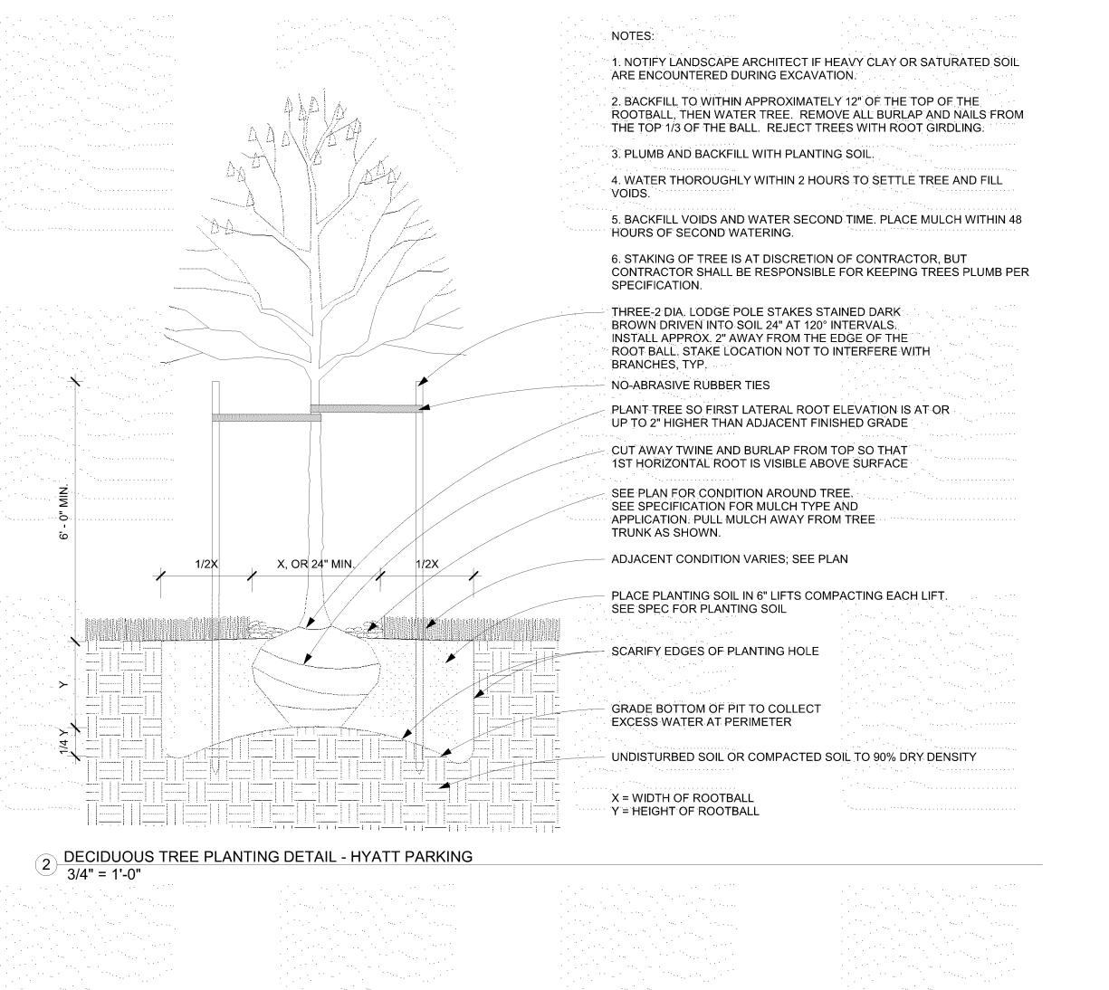
NOTES: 1. NOTIFY LANDSCAPE ARCHITECT IF HEAVY CLAY OR SATURATED SOIL ARE ENCOUNTERED DURING EXCAVATION. 2. MULCH PERFECTLY ROUND MULCH BEDS TO DRIPLINE OF TREE TYP. 3. STAKING OF TREE IS AT DISCRETION OF CONTRACTOR, BUT CONTRACTOR SHALL BE RESPONSIBLE FOR KEEPING TREES PLUMB PER SPECIFICATION.
