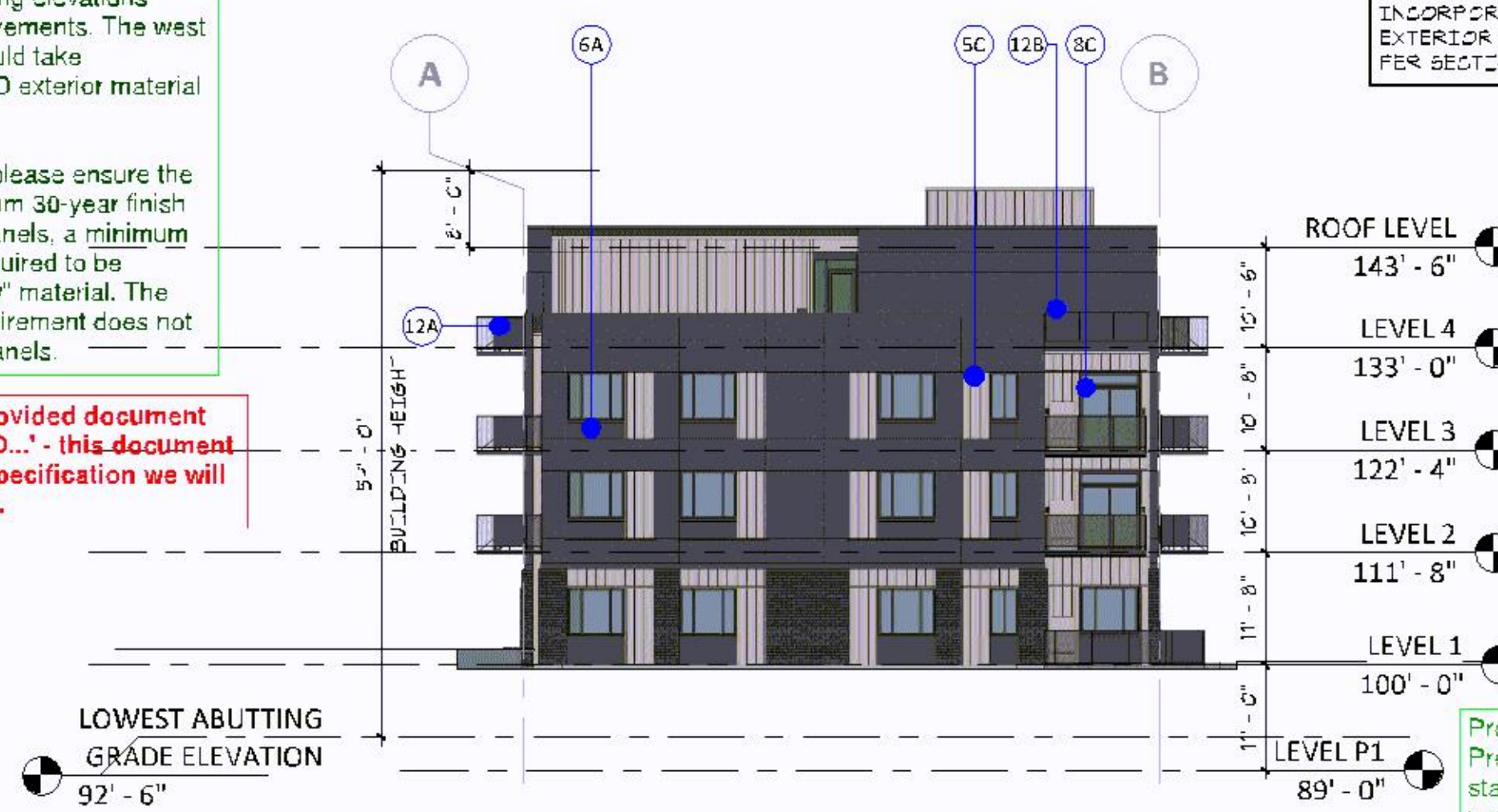
3 WEST ELEVATION DRC-2.1 1/16" = 1'-0"
