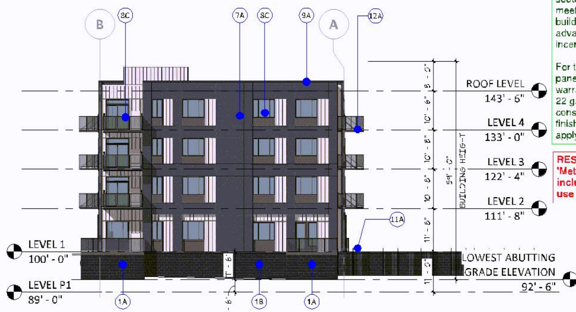
4 EAST ELEVATION DRC-2.1 1/16" = 1'-0"
