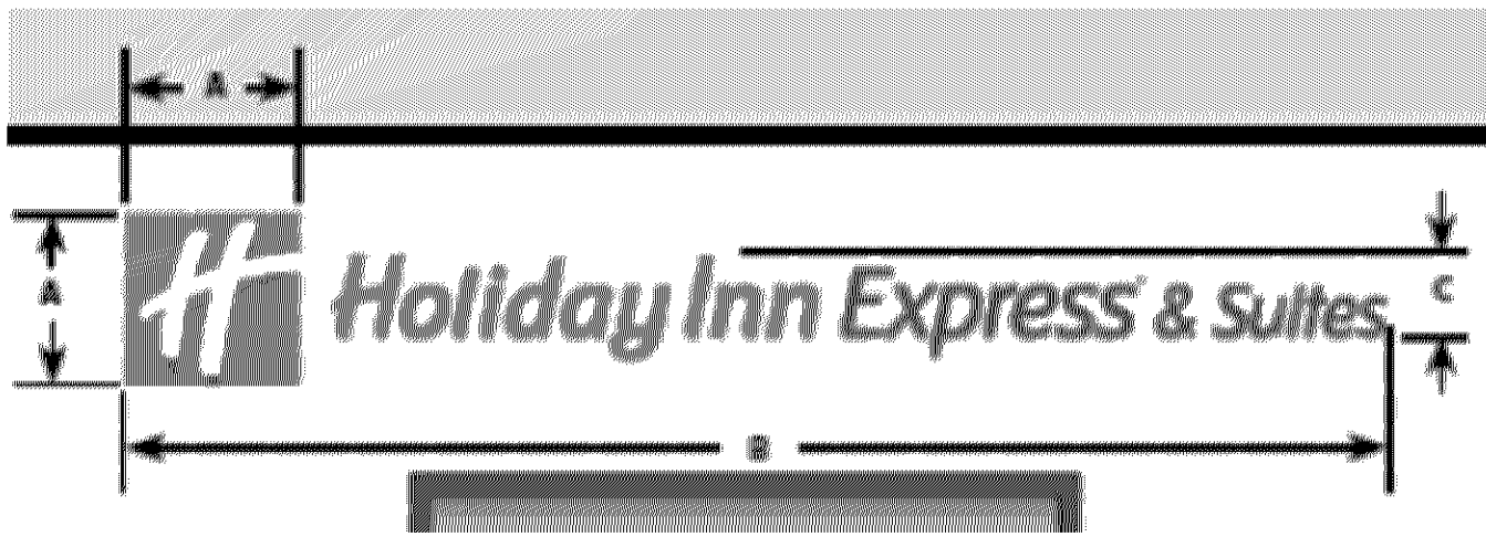
LARGE STRAIGHT WALL SIGN (DLS-LM-6) SIGN AREA = 126 SF (ALLOWED 250 SF MAX) HEIGHT TO TOP OF SIGN = 56'-4" SIGN DIMENSIONS: A = 6'-1 1/2" B = 45'-3" C = 3'-0"
