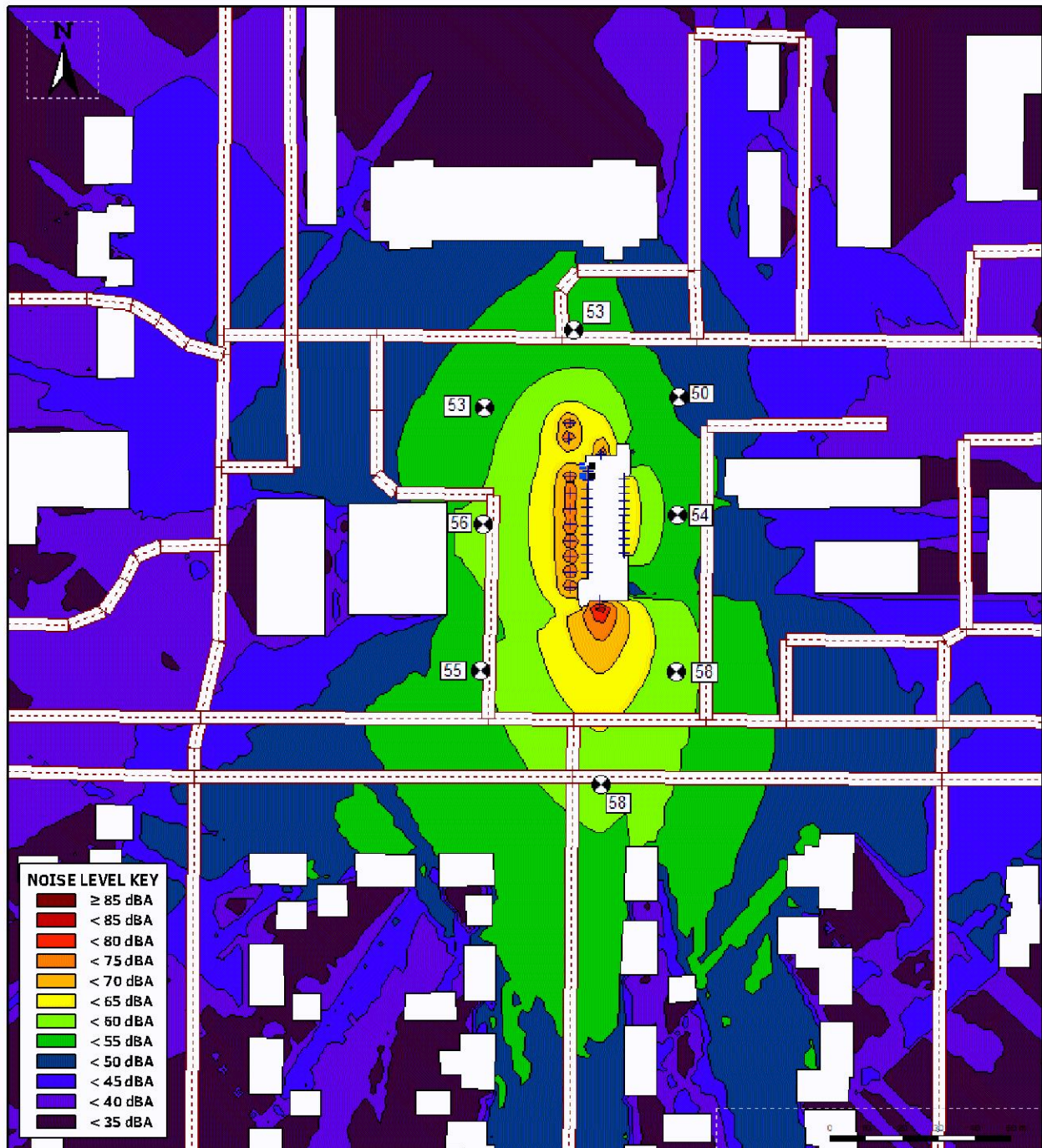
Figure 11 – Noise contour plot showing the Tommy's Express Car Wash equipment noise levels at the proposed Bloomington site with the recommended vacuum mufflers included and the blowers running at 30 Hz.
