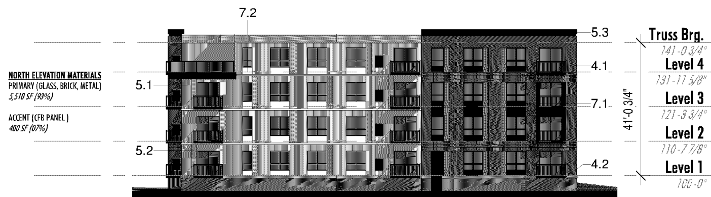
3 Exterior Elevation - North 1" = 30'-0"
