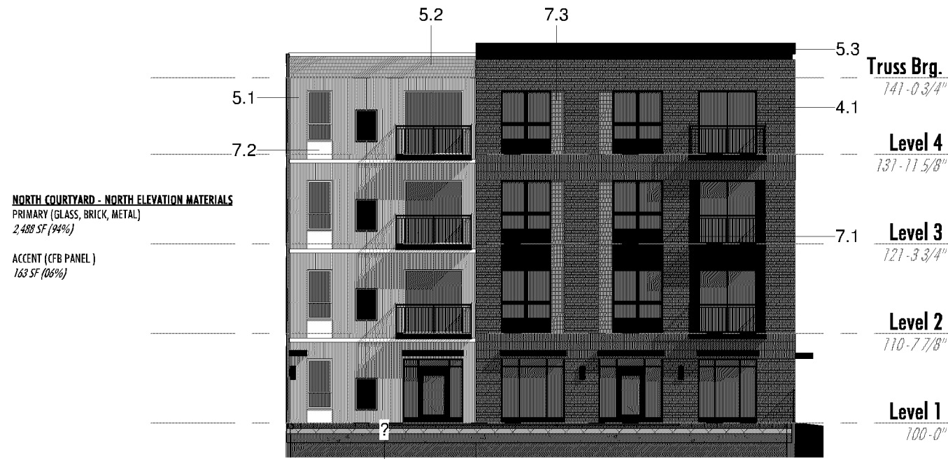
1 Exterior Elevation - North Courtyard (North Facade) 1/16" = 1'-0"
