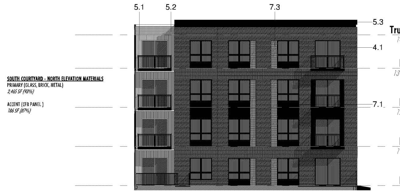
3 Exterior Elevation - South Courtyard (North Facade) 1/16" = 1'-0"
