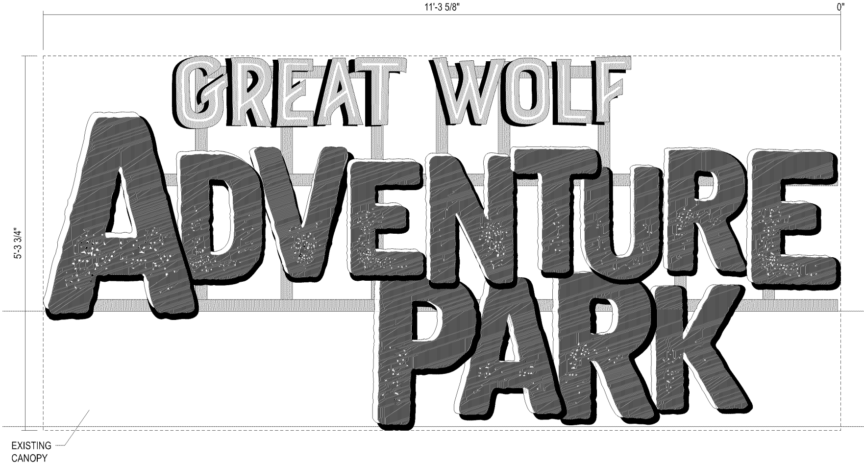
E8 FRONT VIEW - INTERNALLY ILLUMIMATED CHANNEL LETTERS - 60 SQ. FT. SCALE: 3/4"=1'-0"
