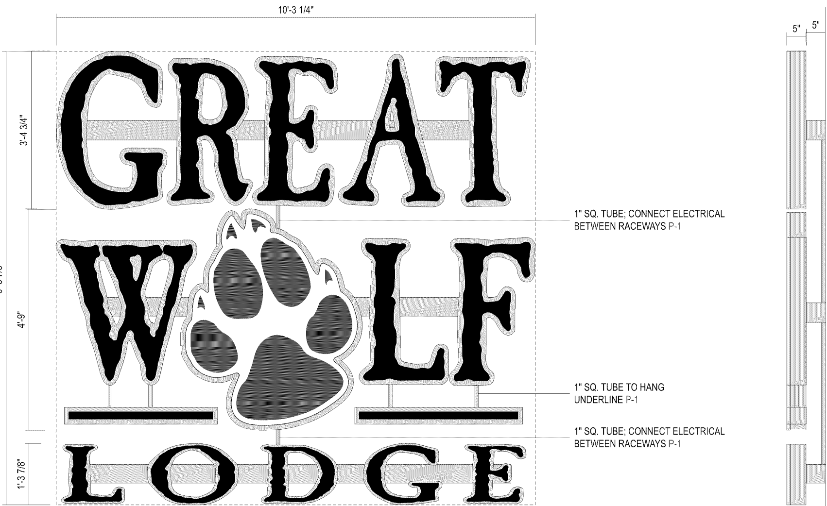
E3 FRONT VIEW - INTERNALLY ILLUMINATED CHANNEL LETTERS - 100 SQ. FT. SCALE: 1/2"=1'-0" SIDE VIEW
