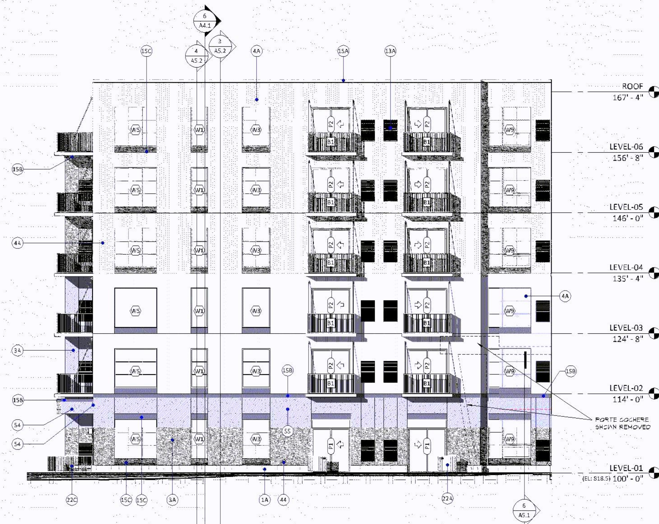
1 COURTYARD A - NORTH ELEVATION A3.3 1/8" = 1'-0"
