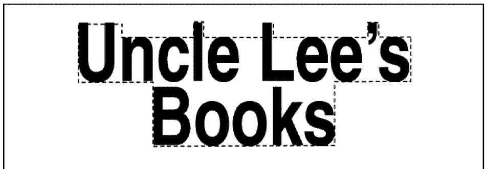
(3) Computation of sign surface area of individual letters mounted on a backer panel.
