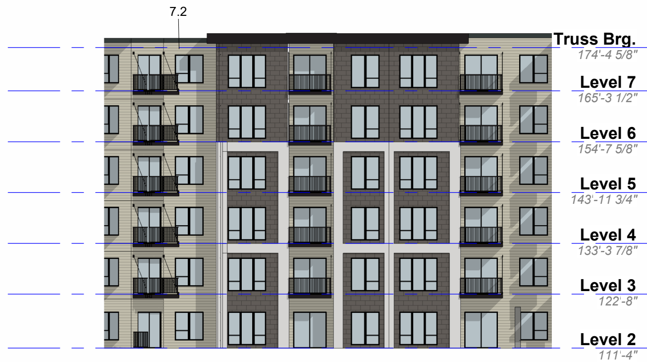
① Elevation - West Courtyard (South Facade) 1" = 20'-0"
