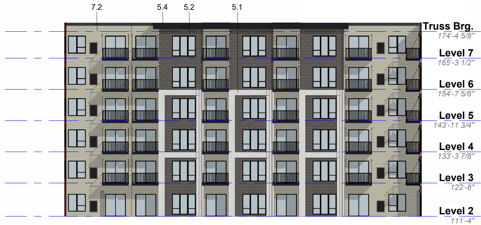
① Elevation - East Courtyard (North Facade) 1" = 20'-0"
