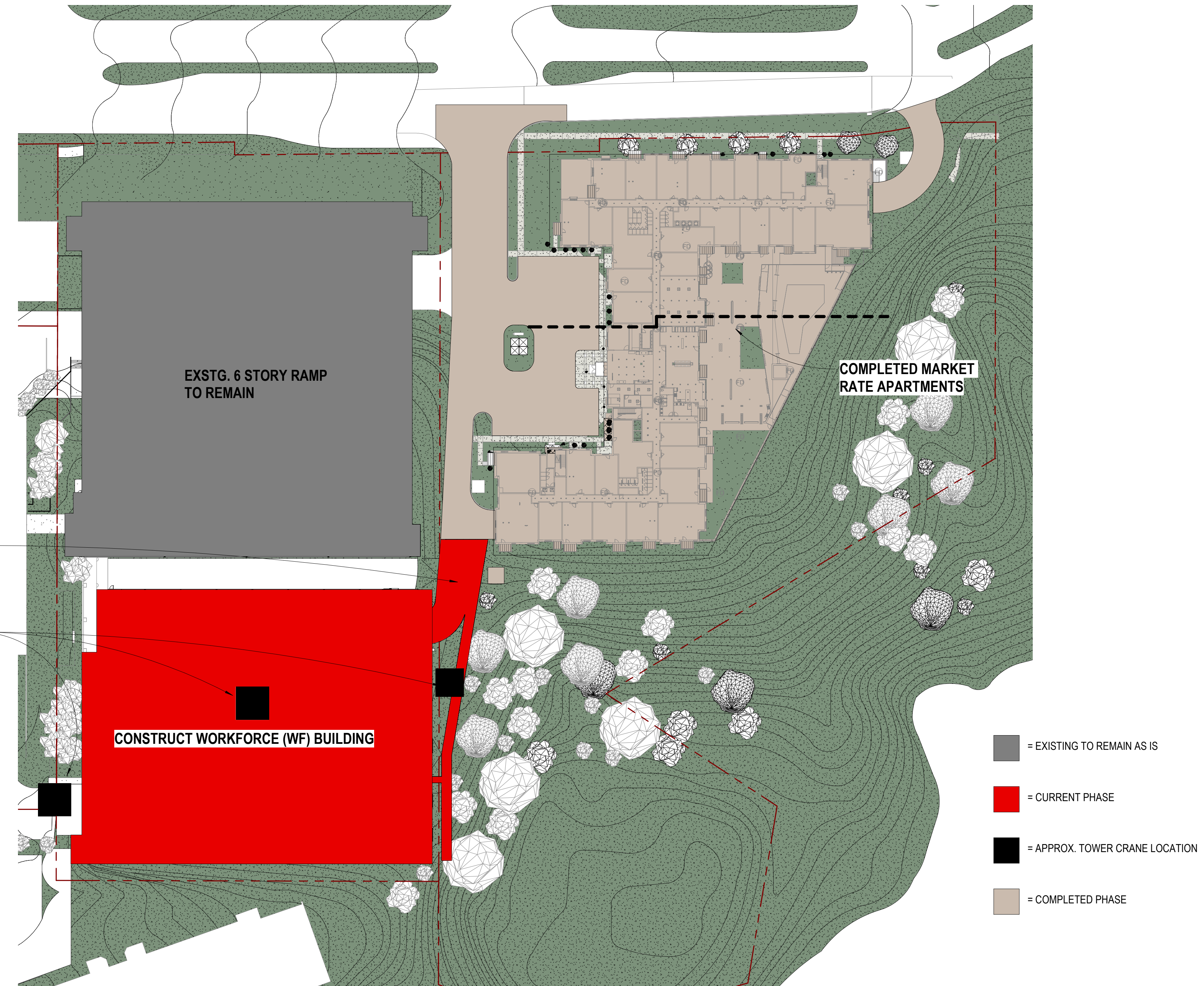
2 PDP CONSTRUCTION PHASING - PHASE 2 SCALE 1" = 50'-0"
