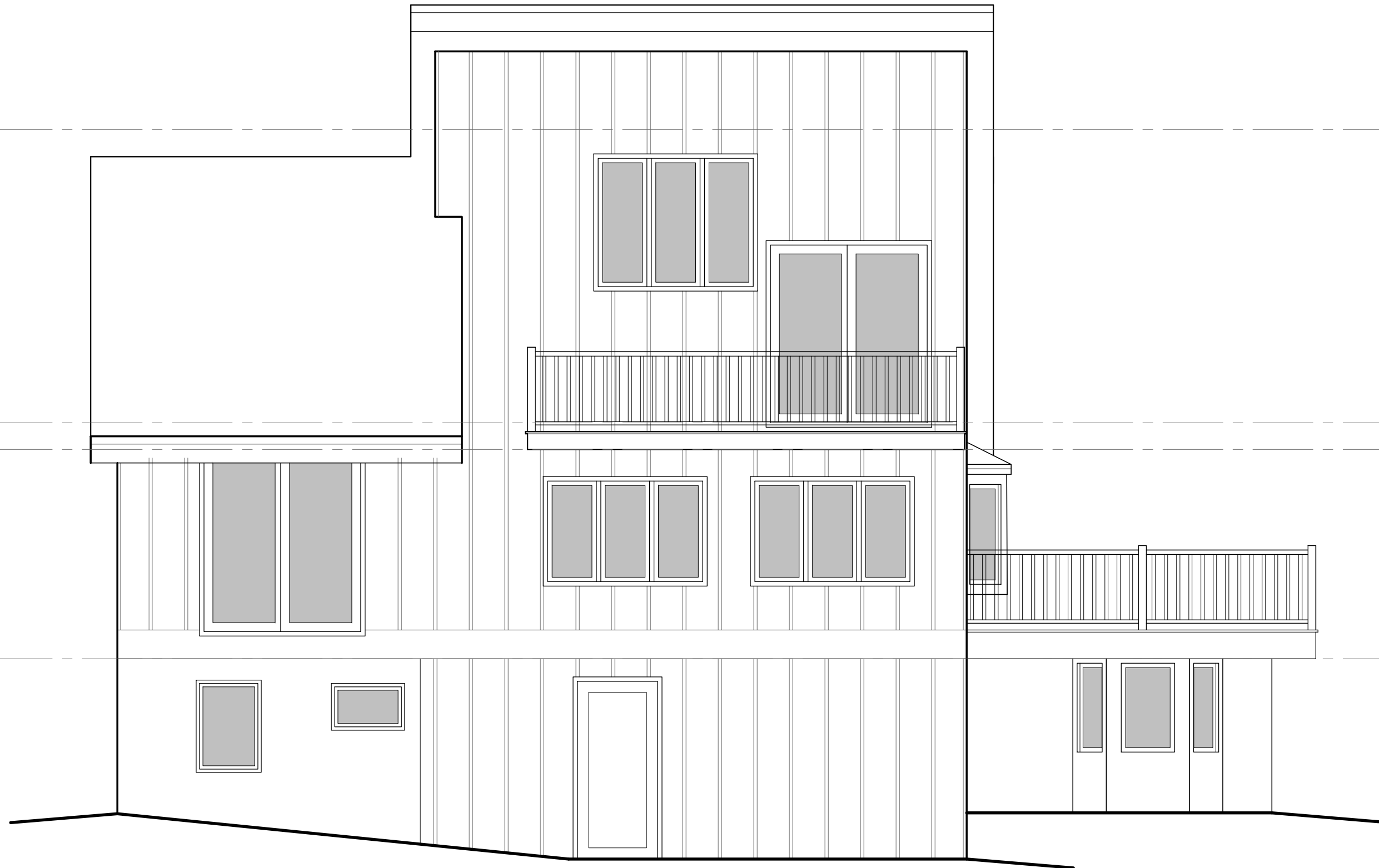
1 Elevations - As-Built Northwest Exterior AB2.2 1/4" = 1'-0"
